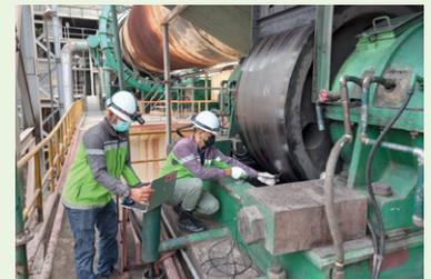
**3. Shell Ovality and Migration:** Check deflection and changes in curvature of shell using Ovality Sensor to prevent cracking and damage to fire bricks inside the machine. Also, check for migration between tyre and shell.
