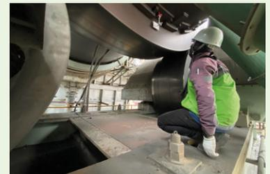
**4. Axial Load Balance:** Check and verify the axial load balance of the machine. And adjust balancing between roller skew load and thrust roller load.
