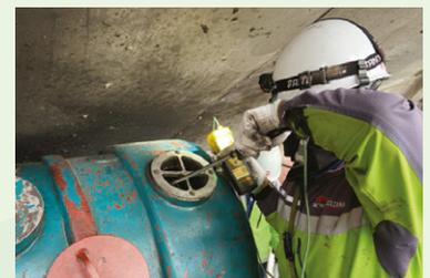
**5. Mechanic Parts:** Check physical condition and measure the dimension, thickness, and deformation of critical components.
