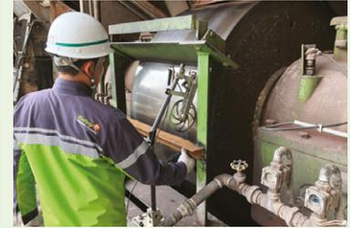
**6. Girth Gear and Pinion:** Check Girth Gear radial and axial alignment, including measure gear tooth temperature profile to verify load distribution.
