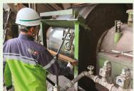
**6. Girth Gear and Pinion:** Check Girth Gear radial and axial alignment, including measure gear tooth temperature profile to verify load distribution.
