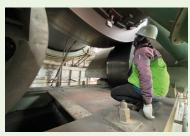
**4. Axial Load Balance:** Check and verify the axial load balance of the machine. And adjust balancing between roller skew load and thrust roller load.
