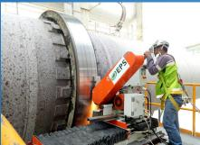
All advanced measurement analysis for the lists as mentioned above shall be carried out by experienced specialist team, during normal kiln operation, with special/ advanced tools & equipment and visual inspection. After that, the follow-up meeting shall be held for the brief of kiln inspection with immediate action recommendations.
